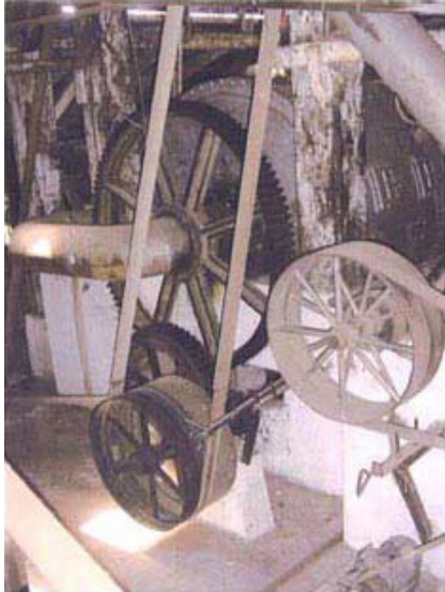
Figure 26. Mechanism of coffee-dryer machine.
