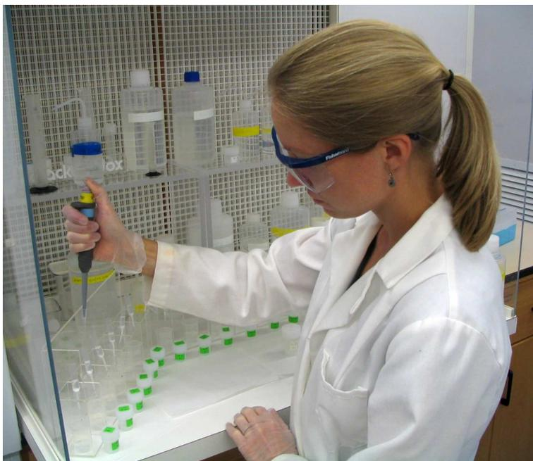
**Figure 16. Loading samples into cation exchange columns packed with strontium resin.**
