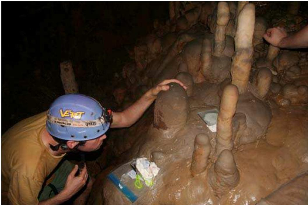
**Figure 21. Drip water collection apparatus being installed at the base of one of the sampled stalagmites.**
