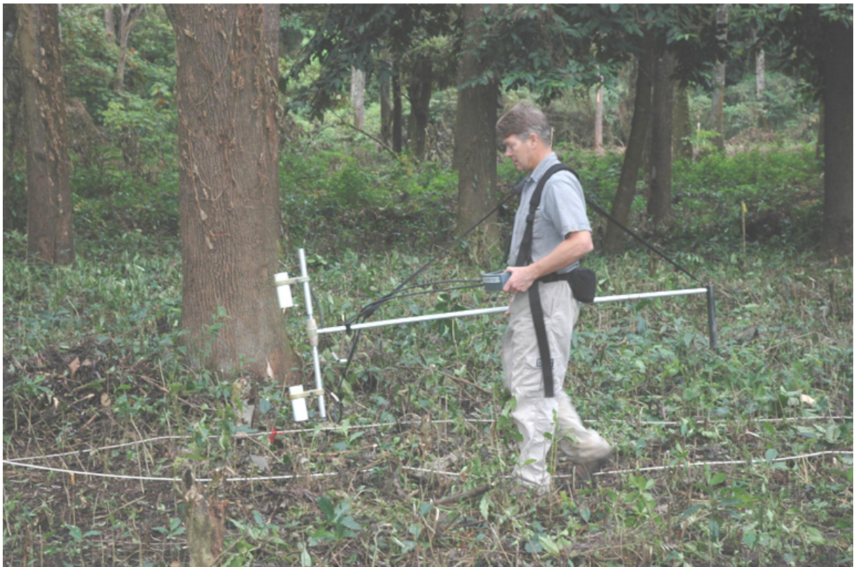
Figure 24. Hector Neff surveying with GPR and magnetometer.
