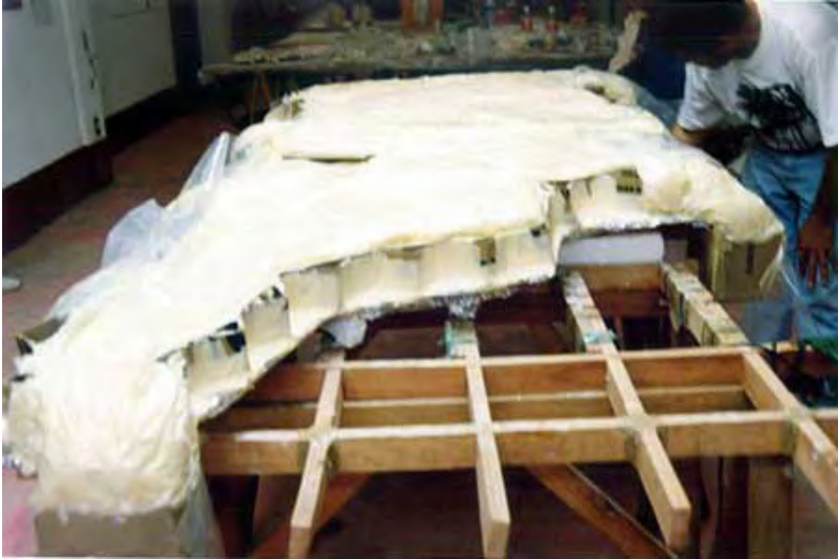
Photo 66. Polyurethane foam layer
