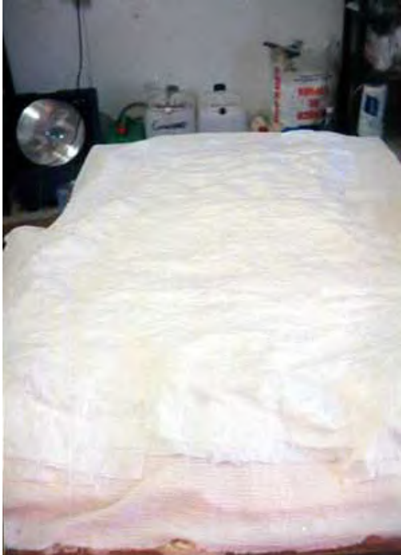
Photo 29. Insulating layers of tissue paper
