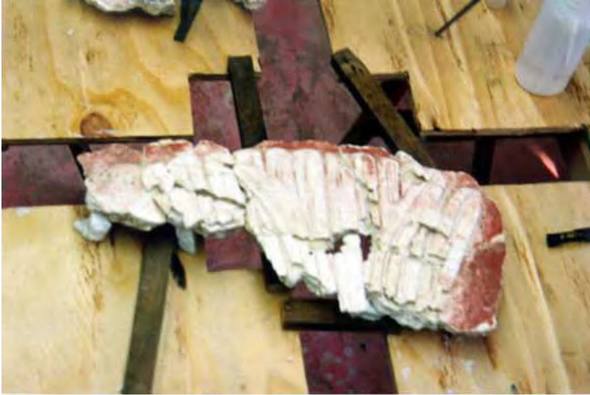
Photo 56. Joining of fragments
