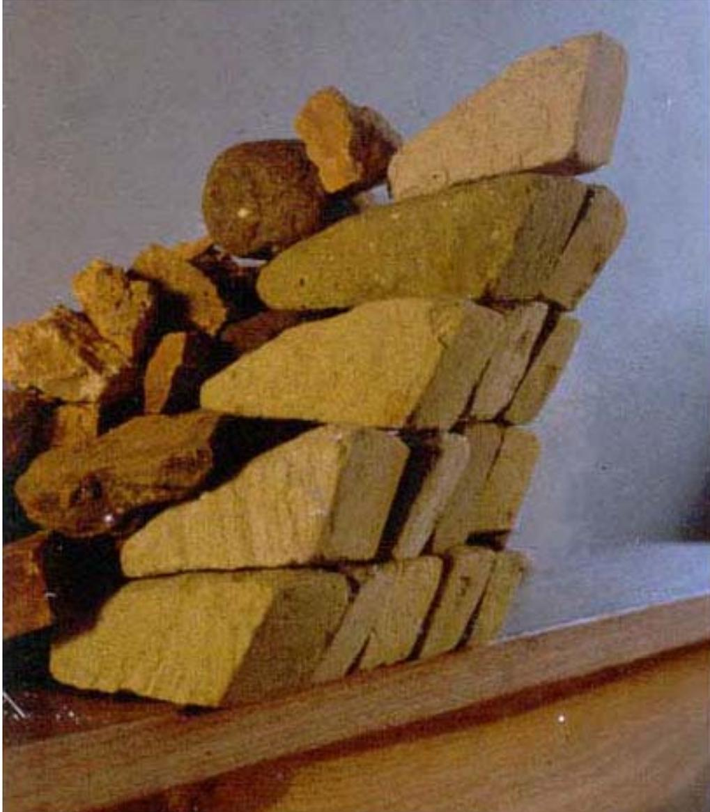
Photo 52. Copán, experiment: scale construction of dry laid vault, October, 1986.
