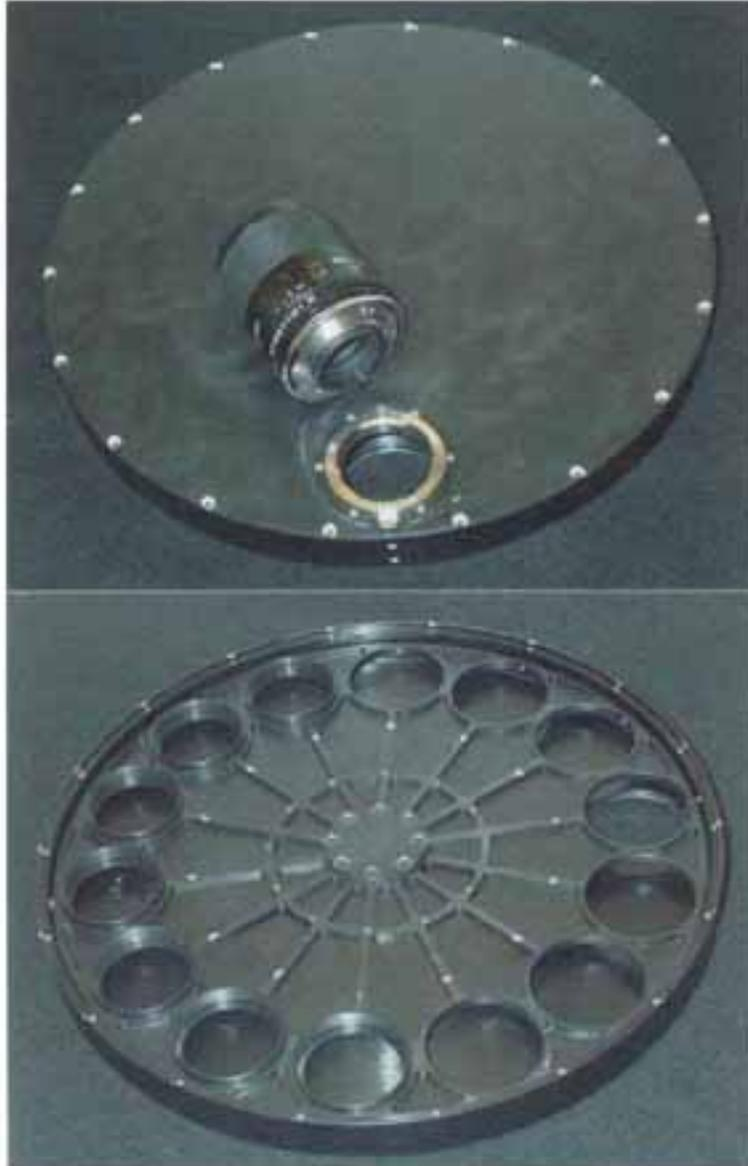
**Figure 5a. Filter wheel and lens (top), and filter wheel interior (bottom).**
