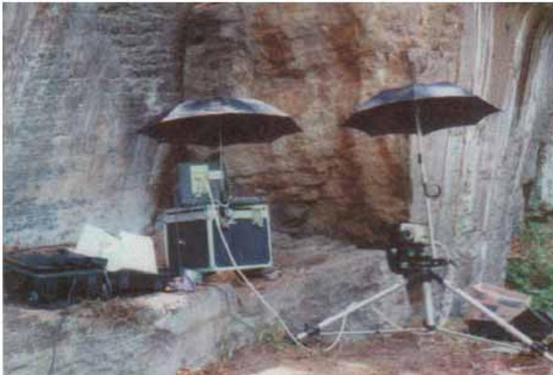
**Figure 1a.** Typical setup of the multispectral imaging equipment at Golondrinas.
