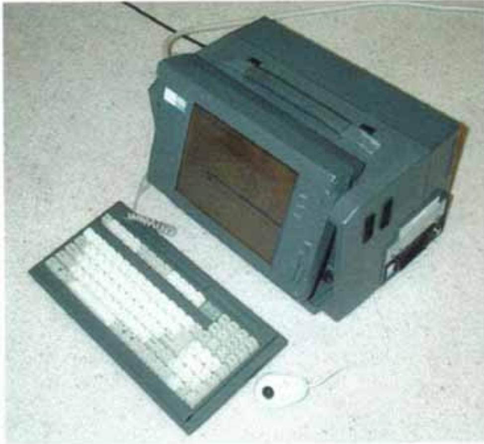
**Figure 7a. System control and data storage computer.**
