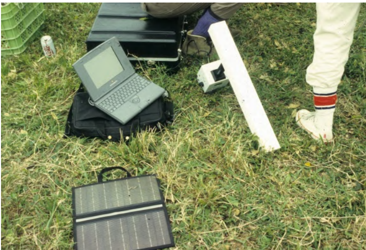
Figure 13.6 Here is the core of the system: the gradiometer Geoscan FM 36, computer, and a power source. Luis' red striped socks are optional, especially in a cattle pasture, but tucking your pants in your socks drastically reduces the number of ticks that find succulent leg and thigh flesh.
