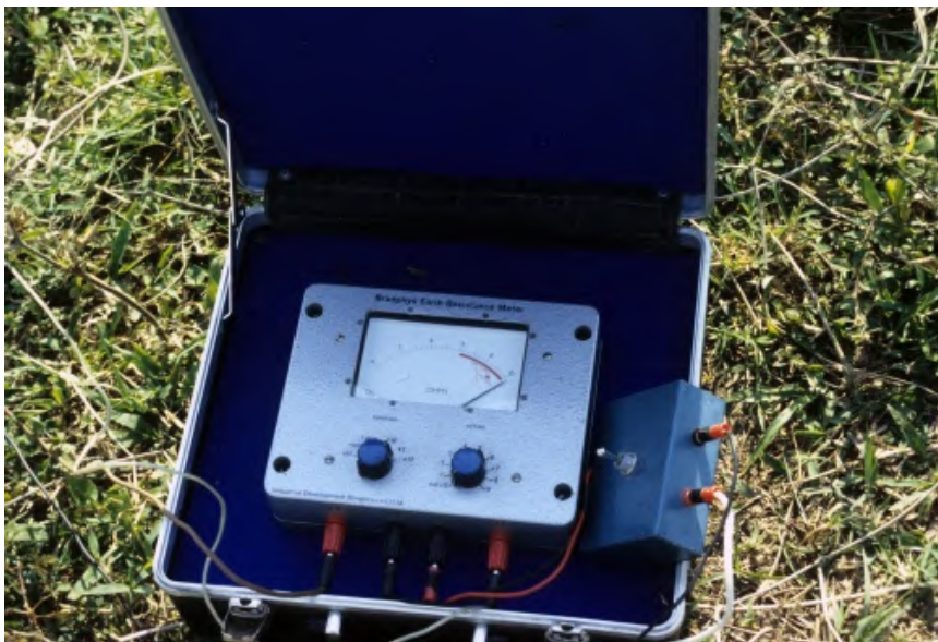
Figure 13.8 The Bradphys IV resistivity meter was specially designed for archaeological work by scientists at Great Britain's University of Bradford, a highly respected center for studies of archaeological prospection.
